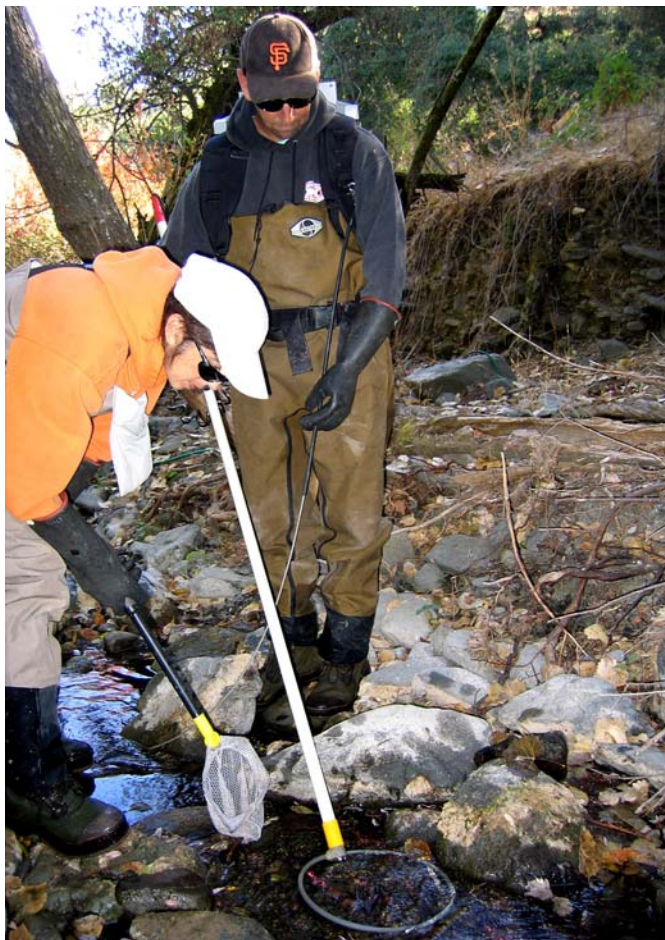
Figure 8-2. SFPUC biologists Patricia McGregor (left) and Pat Conroy electrofishing a low gradient riffle on La Costa Creek.
